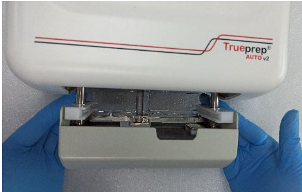
Figure 15: Replacement of discarded Replaceable tray with new
