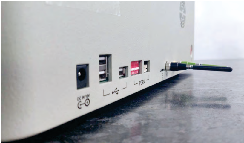
Figure 3: Antenna insert direction
