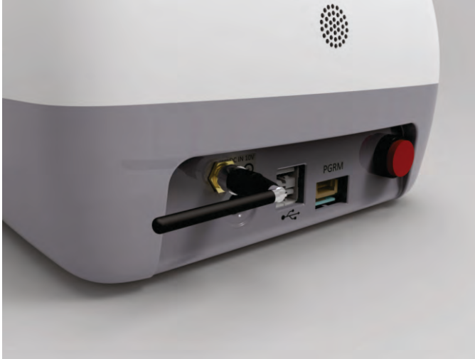
Figure 4: GSM Antenna Position
