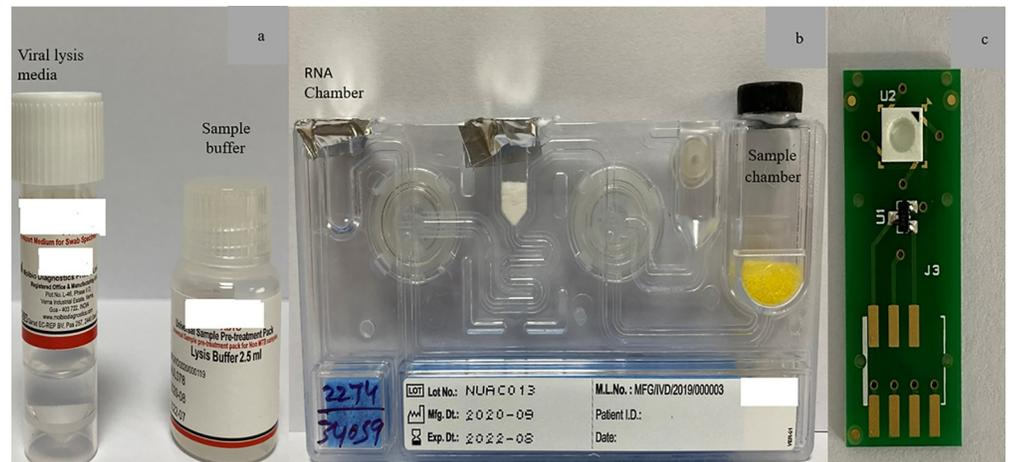
**Fig 1. Heading: Images of consumables used in the TrueNat assay.** Legend: (1a) Viral Lysis media and the sample buffer. (1b) RNA extraction cartridge. (1c) Micro PCR chip.
