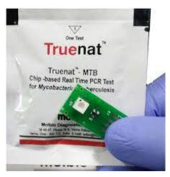
**Fig. 3:** TrueNat MTB chip (Reprinted from molbio diagnostics product listing https://www.molbiodiagnostics.com/product\_detai ls.php?id=1)
