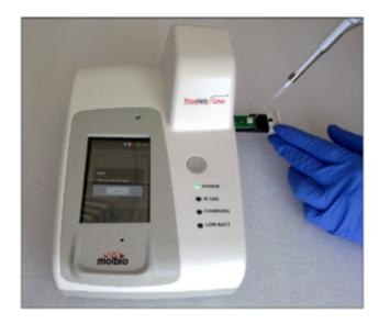
**Fig. 1:** TrueLab PCR analyser (Reprinted from Reprinted from molbio diagnostics product listing https://www.molbiodiagnostic s.com/product\_details.php?id=1)
