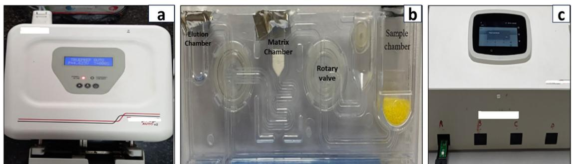
**Figure 2.** Extractor and Micro-PCR devices. (a) TruePrep auto extractor device used for the RNA isolation, (b) cartridge where the blood samples are processed and RNA isolated from blood and (c) Chip-based RT-PCR where  $6\text{ }\mu\text{L}$  of RNA was loaded on Chip for quantification.
